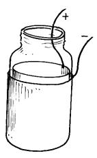
A Leyden Jar, consists of a piece of foil wrapped around the outside of a glass jar, and another piece of foil lining the inside of a glass jar. The energy stored in a charged Leyden Jar is actually stored:A) On the metal foil inside the jar.B) On the metal foil outside the jar.
