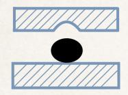
One flange with a semicircular groove done with a rounded mill of the same diameter of the indium wire, machined to a depth equal to half the indium wire diameter. And, the other flange a polished surface.
